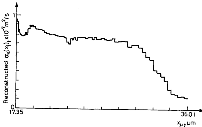
Fig 6 Reconstructed thermal diffusivity depth profile of a 8CB sample at 37.5° in the nematic phase with an applied transverse magnetic field B = 1.65 kG [from Ref. 50]
